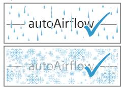
Condensation runs through the condensation channel into the drainage hole to the evaporation pan and does not have to be wiped away. To ensure that the condensation can drain and odours do not form, observe the following information:  $\rightarrow$  "Cleaning the condensation channel and drainage hole", Page 21.
